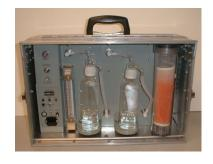
Air sampling around nuclear establishments and from discharge and vent stacks
